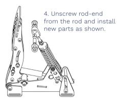
Note: you must re-use the thickest black washers. You can discard the thinnest black washers. These are replaced by a shim on one side and a disc spring on the other side.
