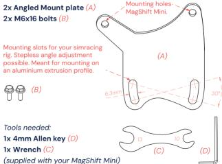
Remove M5 screws on desired\* side of the MagShift Mini with 4mm Allen key supplied with the MagShift Mini.
