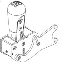
In order to install the mounting plate to an aluminium profile, you can use the M6x16 bolts – supplied with this mount – and the 2x t-nuts\*. Tighten with the wrench.
