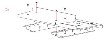
Metal spacers are included with your Baseplate, which you can use to increase the height of the heel plate. For this, use the M5x30 countersunk bolts instead.
