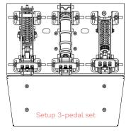
It is advised to connect the pedals to the SmartControl box after installing the pedals but before mounting the Baseplate to your rig.
