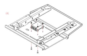
To mount the assembly to your aluminium rig, use the hexagonal bolts M6x12 and M6 t-nuts. For installation on other types of pedal plates use the M6x25 bolts and M6 flanged nuts.
