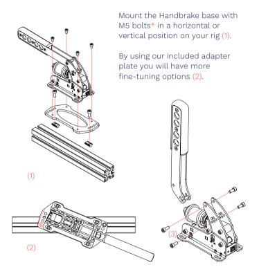
The lever of the Handbrake can be mounted in a horizontal (default) or vertical position relative to the base (3).
