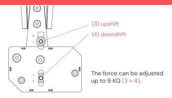
Insert 2 torx keys (5) simultaneously into adjustment bolts (one on each side).
