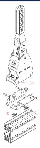
Attach the U-bracket to your simulator (1). The bracket allows for adjustment of the yaw angle.
