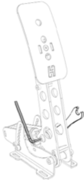
Location of the pedal force curve adjustment bolt.
