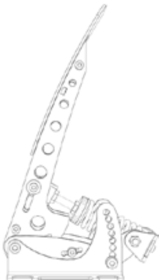
Step 2: Slide the adjustment bolt (shown here in the highest position).
