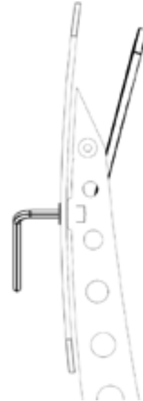
Step 3: Loosen the nut and bolt so the pedal plate can rotate.
